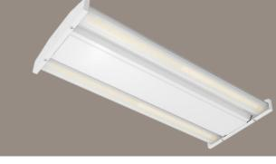
The Trinity Series industrial fixture is a linear highbay series by Aeralux. It is offered in several sizes and has several mounting methods to suit your project space. One of the distinctive feature of this fixture is the use of aluminum extrusions in order to offer the maximum surface area for the heatsinking of the led arrays. This ensures longer lifetime of the fixture while enabling a higher performance.
