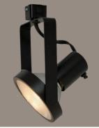
AEH-GBP38 has 2-plane gimbal design that allows 360° horizontal swivel and 150° adjustability in the vertical plane for excellent aiming. "Sure-Set" yoke holds the fixture firmly in place. Integral ON/OFF switch and track polarity indicator are standard.
