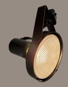
AEH-GFP38 has 2-plane gimbal design that allows  $360^\circ$  horizontal swivel and  $150^\circ$  adjustability in the vertical plane for excellent aiming. "Sure-Set" yoke holds the fixture firmly in place. Integral ON/OFF switch and track polarity indicator are standard.
