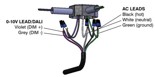
Note: For non-dimming, 3-conductor cord is available (upon request).
