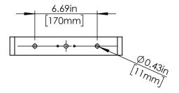
2. Use typical anchor bolts similar to the recommended in size and length. Install anchor bolts according to the anchor bolts installation instruction.
