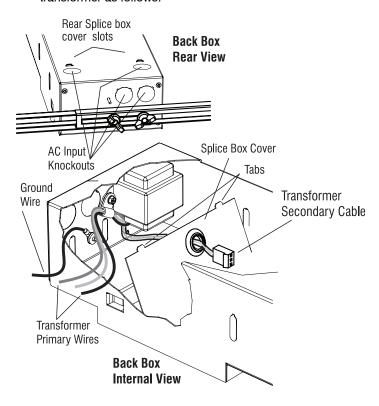
Black lead for 120V or Orange lead for 277V (cap unused lead)
