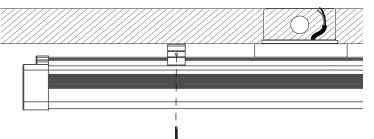
Secure mounting clips to the ceiling Secure canopy to j-box with cross-bar Adjust cord length, do wiring connection Snap in the fixture to the mounting clips
