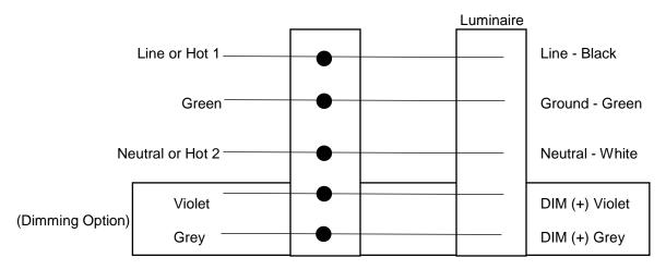
For 16/4 both circuits must be connected to the same branch circuit, i.e. turning off the branch circuit protection will turn off both circuits of the luminaire.
