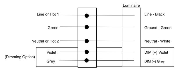
For 16/4 both circuits must be connected to the same branch circuit, i.e. turning off the branch circuit protection will turn off both circuits of the luminaire.
