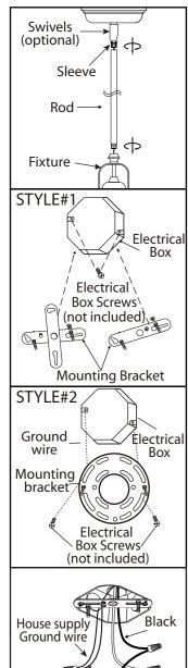
$\mathbb{1}_{\circ}$  Install the length of rod that is required by threading wire through the rod and screwing it to the fixture. Install swivel to the rod, ensuring that the sleeve is at the swivel.
