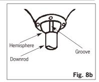
**NOTE:** When installing fan on sloped ceiling, make sure tab on hanger bracket faces towards the top of the slope. Depending on the slope, a longer downrod may be required to prevent fan blades from hitting the ceiling.
