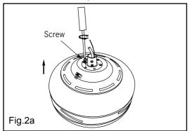
Attach the blades to the fan motor assembly using the screws, metal washer and fibre washer. Slightly turn the blade after installation and repeat the same step for the other blades.
