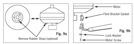
NOTE: Fan comes with three rubber stops (optional on some models) on motor for shipping purposes only. Remove stops before running motor or installing blades to motor.
