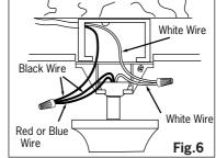
Connect white wire from outlet box to white wire from fan using marret (not supplied).
