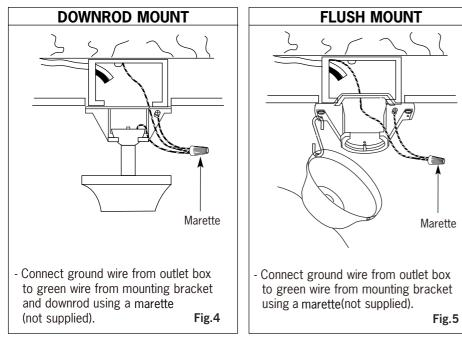
**NOTE**: Once ground wires are connected, carefully tuck wires and marette into the outlet box making sure that the wires are clear of the hemisphere and downrod when positioned in mounting bracket (Downrod Mount Only).
