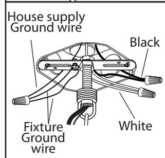
6. Connect the ground wires (bare copper or green) from your fixture (bare copper or green) or ground screw in the electrical box. Connect the black wire (or wire marked "SPT-1") from the fixture to the black wire in the electrical box and connect the white wire (or the wire with ribbed side) from the fixture to the white wire in the electrical box.
