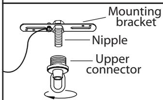
2. Determine the height that you would like to hang your fixture. Trim the cord and chain. Allow 10" of extra wiring for the electrical box connections.
