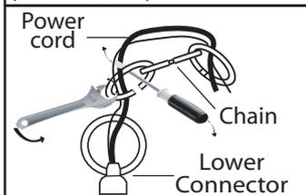
4. To attach chain loop to light fixture, use a screwdriver and wrench to open and close chain loop. Ensure to close the opening. Weave the power cord and ground wire through the links in the chain.
