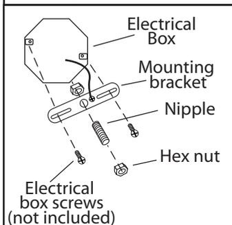
3. Loosen the upper connector from nipple. Attach the mounting bracket to the electrical box using electrical box screws (not included). Attach the nipple to the mounting bracket and adjust until it will clear the canopy when assembled (Place the canopy over the nipple and tighten the upper connector onto the nipple until snug. The upper connector should hold the canopy snug to the ceiling). Lock the nipple in the correct position using the hex nut.
