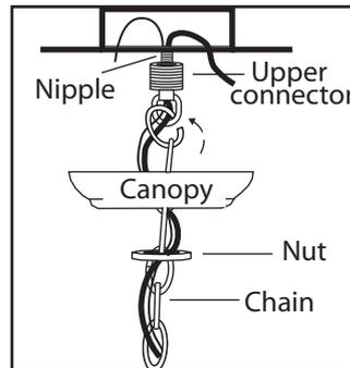
5. Loosen the nut on the upper connector and slide it down the chain towards the lower connector. Slide the canopy down the chain towards the lower connector. Feed the wire through nut, canopy, the upper connector and onto the nipple. Tighten the upper connector onto the nipple. Spread the other end of the chain open and fasten to the upper connector. Ensure the opening is closed.
