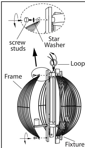
1. Tighten the loop to the stem on the fixture. Install the decorative frames with star washers and screw studs.
