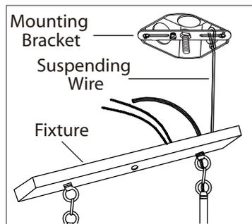
4. Use the suspending wire to hang the fixture as shown for wiring connection.
