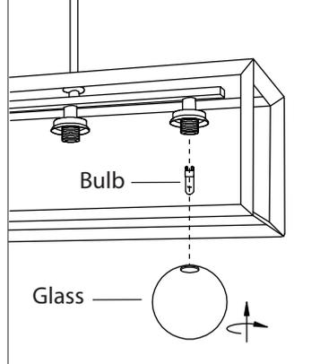
8. Install specified bulb type and wattage (not included). (FROST bulb gives better effect on the glass.)
