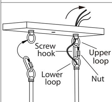
2. Un-Screw the screw hook and insert the upper and lower loop into the screw hook.
