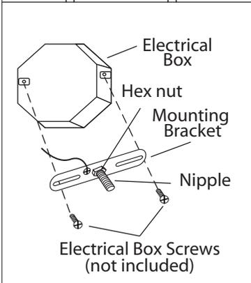
3. Attach nipple to mounting bracket. Adjust so it will clear hole in back of fixture and then lock nipple in place with star washer and hex nut. Attach mounting bracket to electrical box with electrical box screws (not included).
