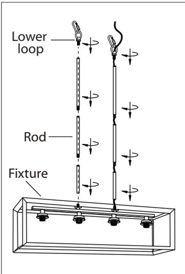
1. Install the length of rod that is required by threading wire through the rod and screwing it to the fixture. Screw the lower loop to the top rod.
