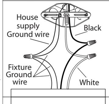
5. Connect the ground wires (bare copper or green) from your fixture to the ground wire (bare copper or green) or ground screw in the electrical box. Connect the black wire from the fixture to the black wire in the electrical box and connect the white wire from the fixture to the white wire in the electrical box.
