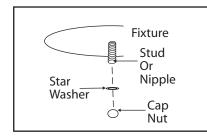
Tuck electrical wires into outlet box and position fixture over studs or nipple on mounting bracket assembly. Secure fixture in place with star washer(s) and cap nut(s).
