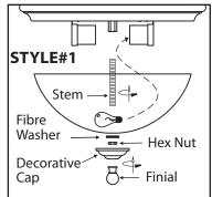
**STYLE#1** - Secure the centre stem onto the screw stud. Install the proper bulb type and wattage. Secure the glass in place using the decorative cap, hex nut, fibre washer and finial.
