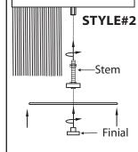
**STYLE#2** -Secure the centre stem onto the screw stud. Install the proper bulb type and wattage. Secure the glass in place by the finial.
