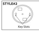
Tuck the electrical wires into the electrical box and position the "key slots" over the support screws. Turn and lock the support screws into the "key slots". Tighten the support screws into place.
