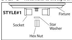
Install the pan through the centre screw stud. Secure the pan using a star washer and hex nut.
