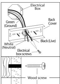
$1_{\circ}$  Feed power cords from the electrical box through the center hole of the back cover. Align holes of back cover over electrical box and secure with electrical box screws (not included).
