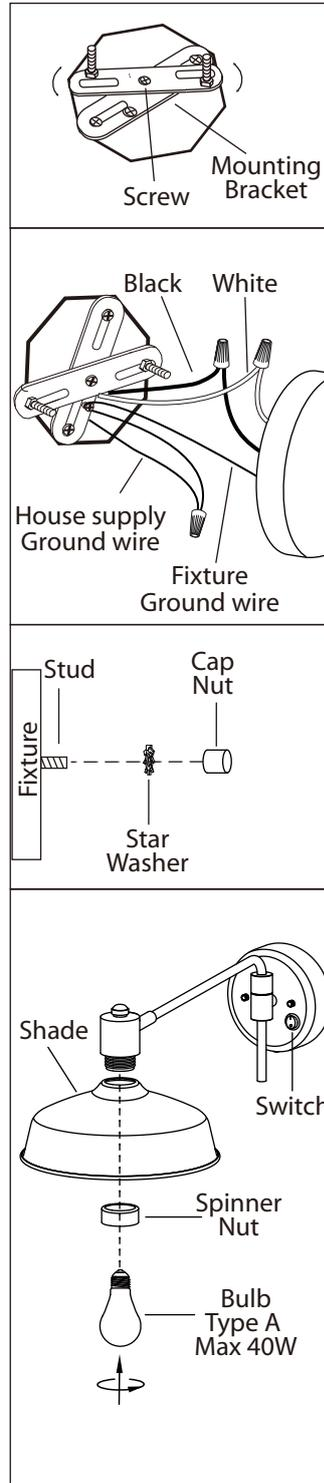
6. Position mounting bracket so that the fixture will be hung properly once it is mounted to the ceiling. Tighten the screw to hold in place.
