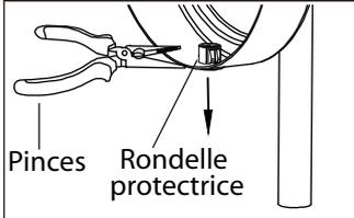
3. Use the pliers to remove the protective ring.
