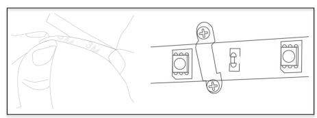
4. MOUNT – Remove the backing to expose adhesive tape. Place in the desired location. To obtain optimum adhesion, ensure the surface is clean. Mounting clips are also provided for extra support.
