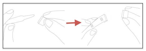
3. CAP – Place a small amount of silicone glue into the end cap, slide cap on to the end of the tape. This will ensure a water-tight seal.
