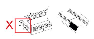
Install all 8pcs of screws for each 4ft fixture. The minimum mounting points required for every 2 or more fixtures are as below:
