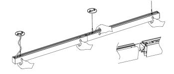
**Note:** Since **18 AWG** wires are used in these luminaires, the max current allowable is **6A**. Please refer to your local electrical code to determine the maximum luminaire allowed on a power line.
