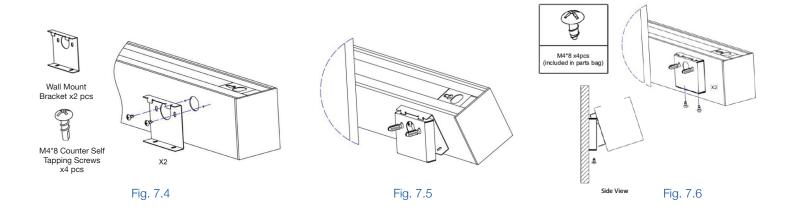
**NOTE:** For continuous row mounting, install connection plates and screws to connect luminaires as per continuous row mounting section "CONTINUOUS ROW MOUNT AND CORNER CONNECTORS". After which, follow the steps shown above to install the wall mount brackets. (Refer to the dimensions below for distance of holes between two luminaires)
