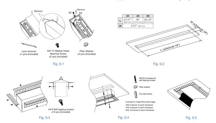
NOTE: For continuous row mounting, install connection kits and screws to connect luminaires as per the section "CONTINUOUS ROW MOUNT AND CORNER CONNECTORS" in the included installation instructions. Then follow the Mud-In Recessed Kit instructions to complete. Do not install the shorter end pieces between every 2 luminaires.
