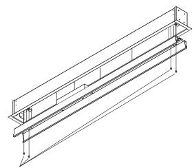
**3.** Remove gear tray assembly from outer shell. Loosen the #8 screws at the locations shown.
