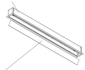
2. Remove lens from fixture and store in secure area.
