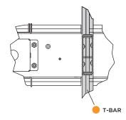
5. Interlock endcap bracket for end to end installation..
