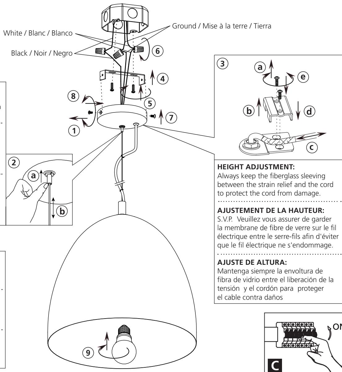
Push the "push-pin" button to release the tension and adjust the height. Once set in desired position release the push pin.
