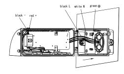
Connect the input wire and the dimming wire of the light, then put the connected wires into the embedded terminal box.
