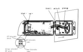
After the wiring completed, set the CCT and power value through the internal switches. According to the label, users can dial the desired color temperature value and power value.
