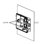
Use screw to lock the lamp base on the embedded junction box.
