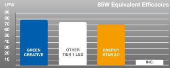
At 79 LPW, this lamp's efficacy is higher than the Tier 1 LED BR40 85W replacement industry average and exceeds the new ENERGY STAR 2.0 requirements. This energy-saving performance makes this lamp a smart retrofit choice for incandescent bulbs.
