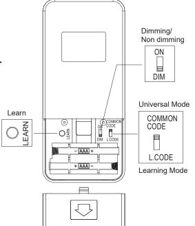
Remote Control Fan Speed And Light Functions.
