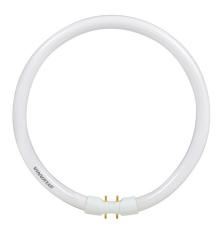
SYLVANIA PENTRON Circline lamps are high lumen output circular shaped T5 diameter lamps that deliver up to 70% more lumens than T9, rapid start Circline lamps. These lamps, available in 9-inch and 12-inch versions, are comparable in diameter to the T9 lamps. The rare earth tri-phosphors are utilized to deliver high lumen output with excellent color rendition and high lumen maintenance.
