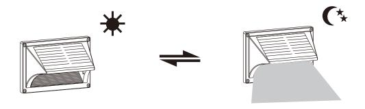
The light is automatically off in the daytime while the solar panel charges.
