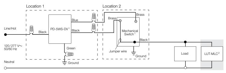
1 Location of Caséta® Wireless In-Wall Switch and mechanical switch may be reversed.
