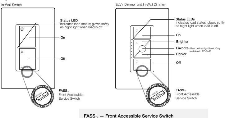
Important Notice: To service load, remove power by pulling out the FASS™ as far as possible. To restore power after servicing load, push the FASS™ back in completely.
