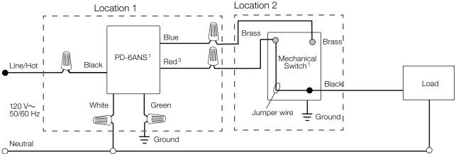
1 Location of Caséta® Wireless In-Wall Switch and mechanical switch may be reversed.
