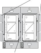
Each Switch/Dimmer has inside fins removed
