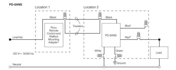
1 When using controls without mechanical 3-way switch, cap the blue terminal. Do not connect the blue wire to any other wiring or to ground. 2
