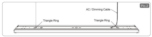
1.) Connect each of the two Triangle Ring on the light fixture to two cables (not included with the product) properly fixed to the ceiling as shown in **Pic.2**.
