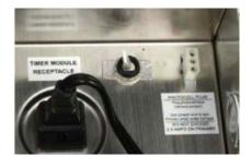
Unplug the jumper connection from the transformer
