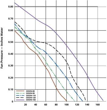
Fan Flow Rate CFM Standard Air
