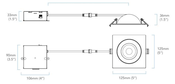
\*NOTE: Width in ceiling needed for the driver to fit is 3" Cut hole size 4-1/4" (108mm)
