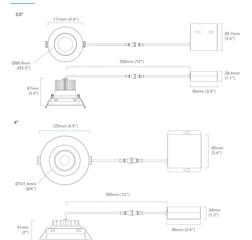
\*NOTE: Width in ceiling needed for the driver to fit is 3" Cut hole size 4-3/8" (110mm)
