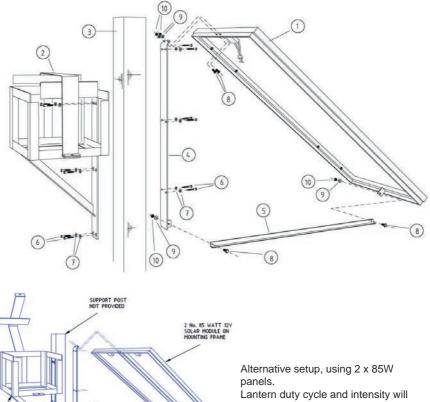
Lantern duty cycle and intensity will determine the size and quantity of solar panels and batteries.
