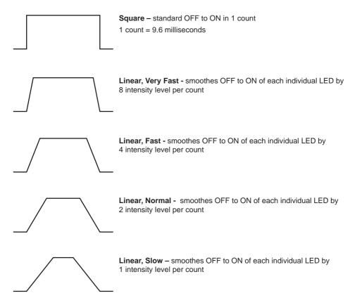
**PLEASE NOTE:** programming the LEDs to have "linear slow" leading and trailing edges is particularly useful for rotating beacons as this emulates a smoother transition from one LED to the next, giving the impression of a mechanical rotating beacon without the drawback of moving parts.
