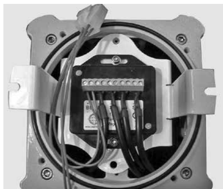
SL10 AMP Regulator shown when correctly fitted
