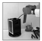
To achieve a satisfactory seal, it is recommended that a torque of 3Nm is applied to the bolts used for holding down the Light Head to the Solar Base and that only the supplied bolts are used.
