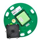
Internal user-replaceable battery in sealed battery compartment
