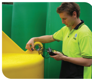
Ultrasonic testing ensures consistency of wall thickness in key areas such as mooring points.
