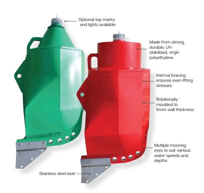
The unique, one piece float section has an internally integrated bow and keel which ensures the buoy remains stable during fast currents. The SL-B750 is rotationally-moulded from UV-stabilised, virgin polyethylene in a range of IALA recommended configurations and colours to ensure clear visibility, and may be fitted with a Sealite LED lantern for safe night navigation.
