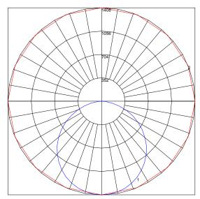
$\label{eq:maximum Candela} \begin{tabular}{ll} Maximum Candela = 1407.6 & Located At Horizontal Angle = 0, Vertical Angle = 0 \\ \# 1 - Vertical Plane Through Horizontal Angles (0 - 180) (Through Max. Cd.) \\ \# 2 - Horizontal Cone Through Vertical Angle (0) (Through Max. Cd.) \\ \end{tabular}$
