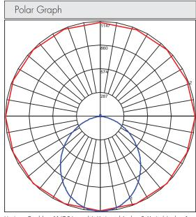
Maximum Candela = 1147.2 Located At Horizontal Angle = 0, Vertical Angle = 1 # 1 - Vertical Plane Through Horizontal Angles (0 - 180) [Through Max. Cd.] # 2 - Horizontal Cone Through Vertical Angle (1) [Through Max. Cd.)
