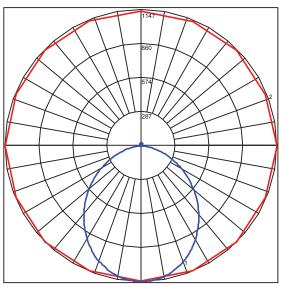
Maximum Candela = 1147.2 Located At Horizontal Angle = 0, Vertical Angle = 1 # 1 - Vertical Plane Through Horizontal Angles (0 - 180) [Through Max. Cd.]
