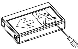
2.Knockout in back of mounting plate and push wires through the hole.
