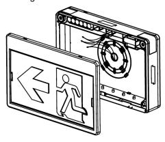
3. Make the proper supply lead connections.
