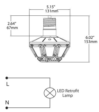
Easy to install - bypass ballast and provide voltage directly to lamp
